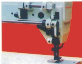
**Three synchronized combined feed mechanism can avoided the slipping between sewing materials.**
