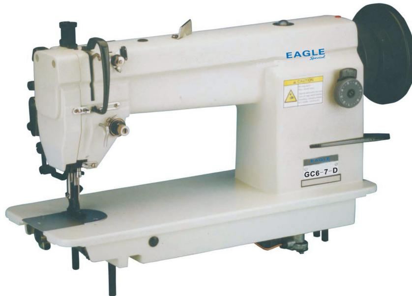
Model GC6-7-D high speed medium and heavy material combine feed sewing machines are the products higher than the model GC6-7 for its new design. The method to feed is the synchronized feed of walking presser foot, needle and feed god. They have the advantages of it's original products and improve the feed mechanism, increase the automatic lubrication device. Sewing performance are better. They are widely used in the factories if suitcase, tarpaulin, cushion, leather goods.
