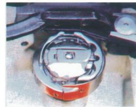
**The using of the big rotating hook reduce to exchange bobbin thread, improve sewing efficiency and increase the lives.**
